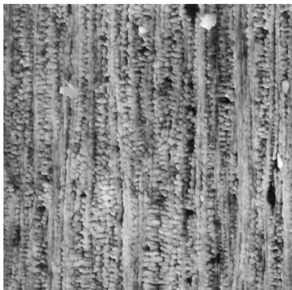
Figure 11 AFM image of the shear region of a SCORIM molding of polybutene-1 (DP4137). The depicted area is 5 \times 5 \mu\text{m} , and the z-scale is 200 nm.
